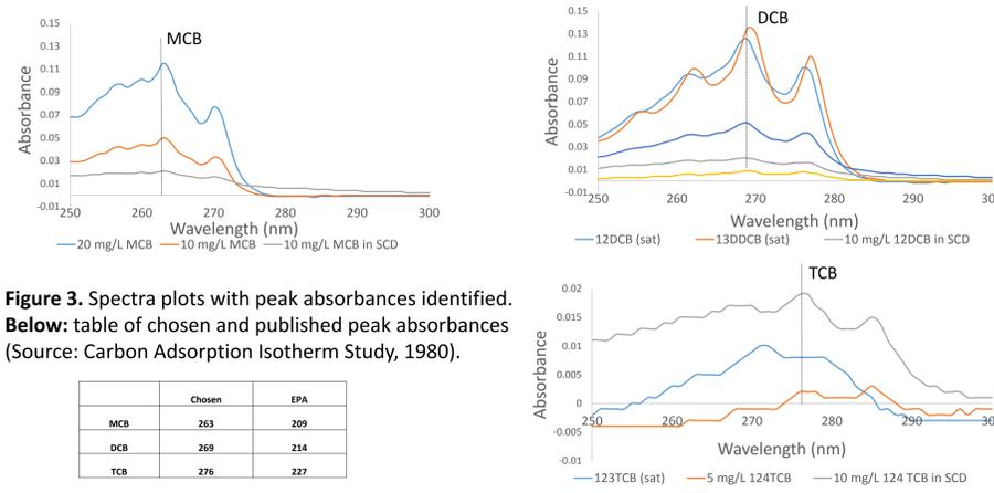
Figure 3. Spectra plots with peak absorbances identified. Below: table of chosen and published peak absorbances (Source: Carbon Adsorption Isotherm Study, 1980).
