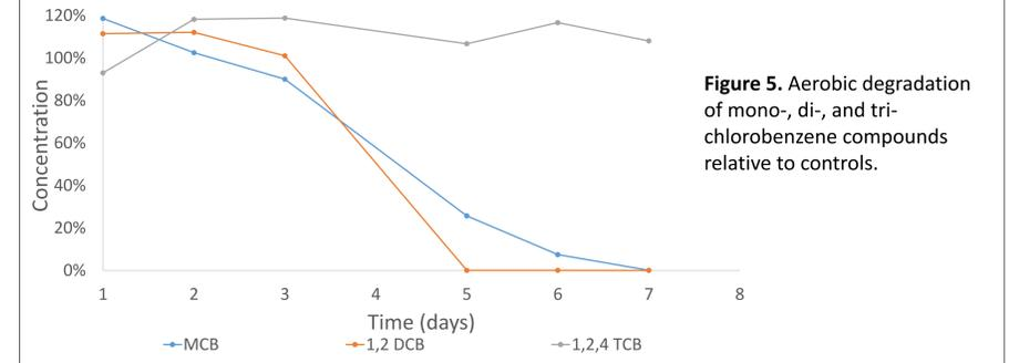
Figure 5. Aerobic degradation of mono-, di-, and tri-chlorobenzene compounds relative to controls.
