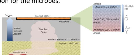
Figure 2. Diagram of the proposed reactive barrier
