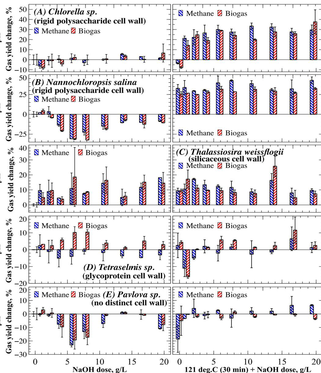
Fig. 3. Influence of thermal, chemical and thermochemical pretreatments on biogas and methane yield
